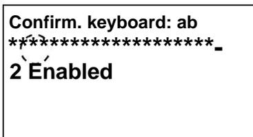
**1 In the Alarm menu screen, press  $\bar{y}$  or  $\bar{y}$  to select Confirm. keyboard.**
